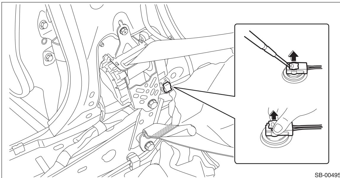
5) Short the alligator clip and terminal of the airbag deployment tool together.
