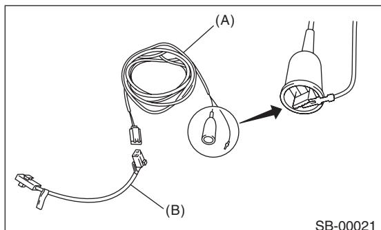
7) Connect the test harness adapter D connector to the pretensioner.
