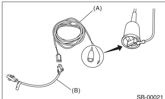
17) Connect the test harness adapter D connector to the lap seat belt pretensioner.
